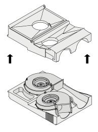
Clean the fans with a soft brush.Make sure the balancing weights do not shift!
