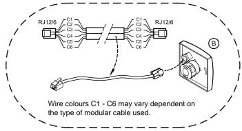
Note: For the modular cable use, the "tab" of both modular connectors must be mounted facing the mark on the modular cable.
