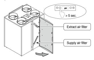
2 Remove the filters. Remember in what way the filters are taken out.
