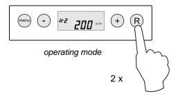
All fault messages can be deleted by pressing the "R" key in the service menu during 5 seconds; This is only possible when there is <u>no</u> active fault!
