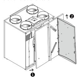
4 Remove the heat exchanger. Be careful not to damage the foam parts in the appliance.
