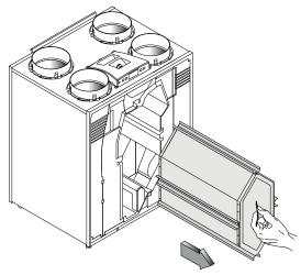
5 Rinse the exchanger with hot water (max. 55 °C) and a regular detergent. Rinse the exchanger with hot water.
