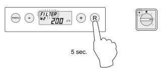
After the filter reset, the text "FILTER"; disappears, the light at the multiple switch is off and the display is back to operating mode.
