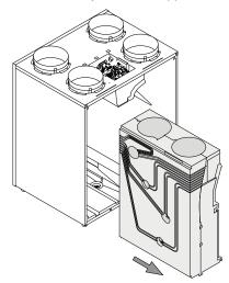
9 Place the fan assembly on a flat surface with the pressure hoses facing up. Remove the red and blue pressure hose without black mark from the pressure tubes mounted in the fan assembly. Turn over the foam assembly so the section with the pressure hoses is facing down.
