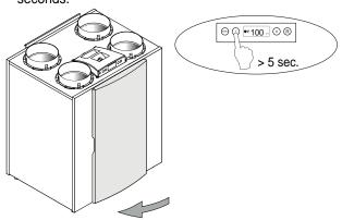
6 After the filters have been cleaned or replaced, press the "R" key for 5 seconds to reset the filter indication.
