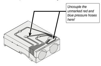
10 Now the fan assembly can carefully be split so the two fans are accessible. Make sure the fans remain in the lower fan section!
