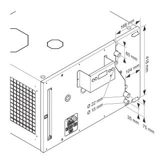
Position of water connection and condensation discharge connection of the right-hand version.
