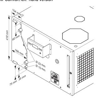
Position of water connection and condensation discharge connection of the left-hand version.
