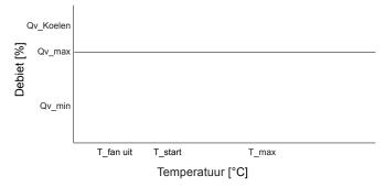
Position 3 - the system ventilator operates constantly at the set air flow for cooling. This can be set with parameter 4.
