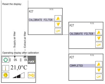
By touching the icon "A", the unit switches to the calibration mode. Display flashes "CALIBRATE FILTER". After calibration, the display shows "COMPLETED". The contamination display is set back to 0% after calibration mode. The filter change counter will then increase by one.
