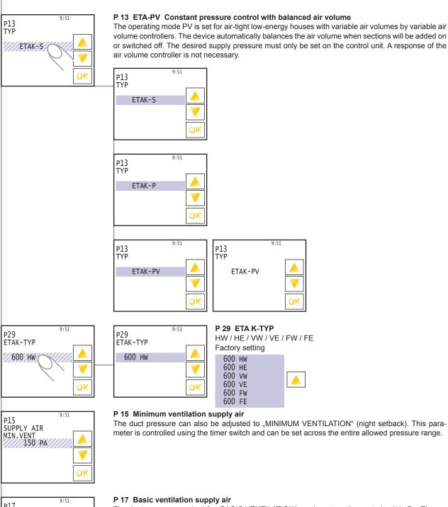
The duct pressure required for "BASIC VENTILATION" can be set on the control unit in Pa. The extract air volume automatically follows up the supply air volume. Expensive control methods can thus be omitted and the air volume balance for the building ventilation can be automatically implemented.
