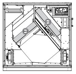
Fig. 24: Position air filter
