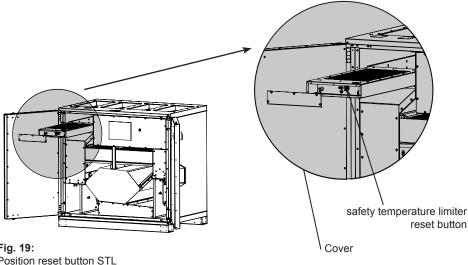
Fig. 19: Position reset button STL ETA K 600 V (1 STB)
